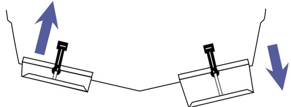
The starboard button controls the starboard tab upwards first and then the port tab downwards.
