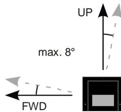
The control unit should be mounted in an upright position. The label on the front side is marked with an UP arrow that should point upwards and a FWD arrow that should point in the forward direction. Exact mounting is not critical, however, as the desired running attitude is set after installation.
