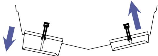
Should the trim tabs move in the wrong direction: For hydraulic trim tabs, exchange the 3 and 4 wires, for electromechanical trim tabs, exchange the 3 and 5 wires with the 4 and 6 wires.
